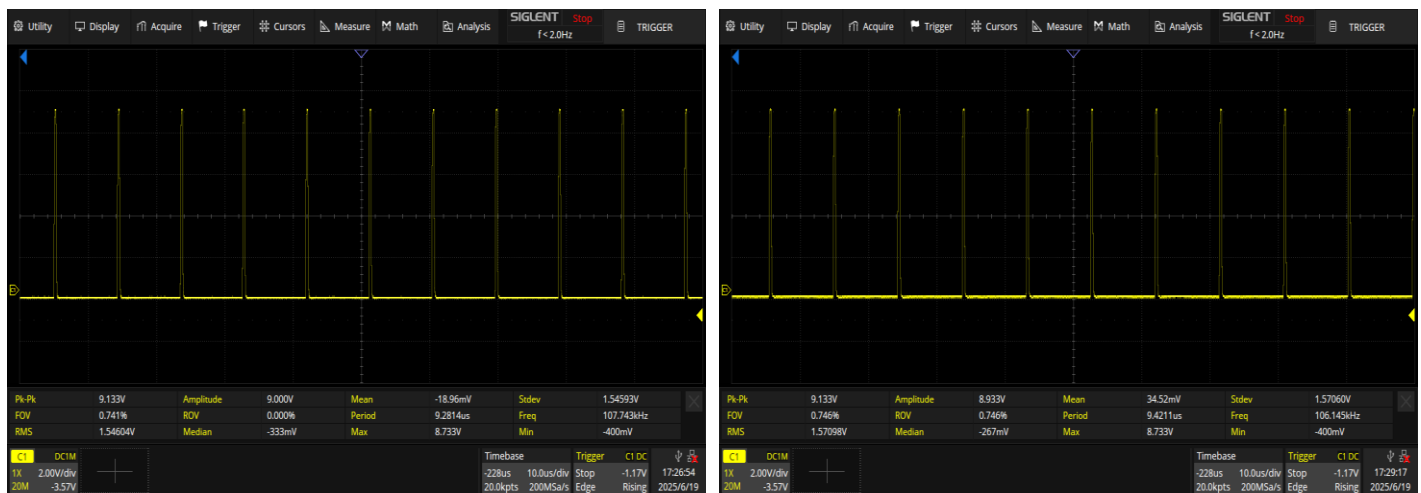
Figure 14 Output frequency of the second detection circuit.
