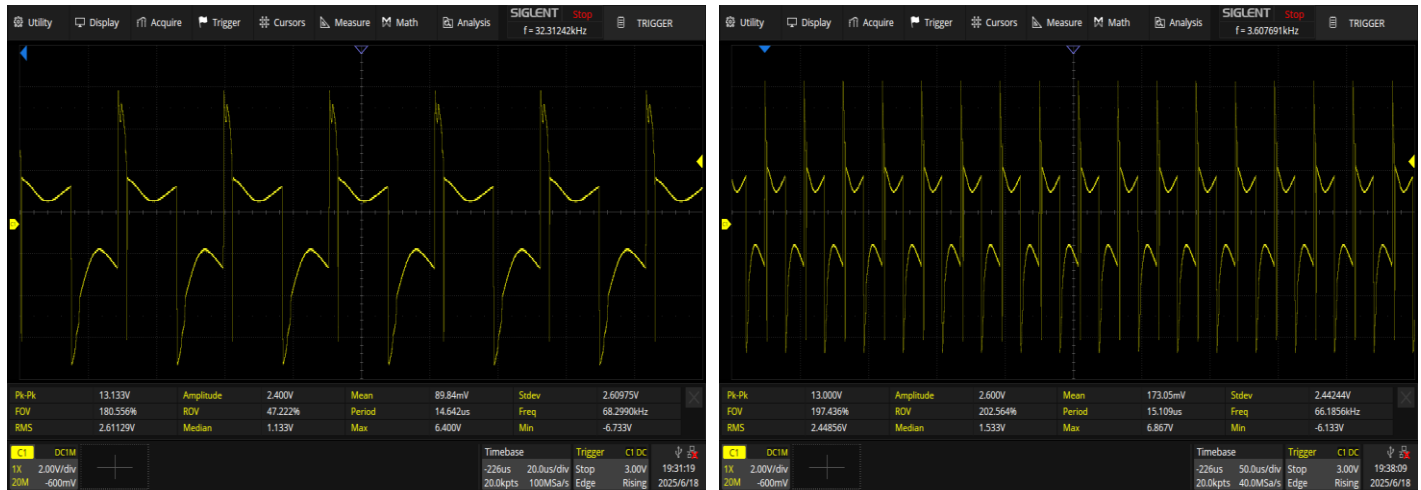
Figure 13 Output frequency of the first detection circuit.
